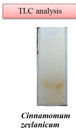
Fig 4: TLC plate. Thin layer chromatography fingerprint of Cinnamomum zeylanicum Aqueous Ethanolic extract.
